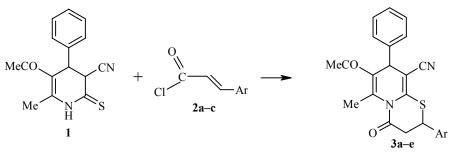
**2**, **3** a Ar = Ph; b Ar = 4-MeOC<sub>6</sub>H<sub>4</sub>; c Ar = 3-O<sub>2</sub>NC<sub>6</sub>H<sub>4</sub>
